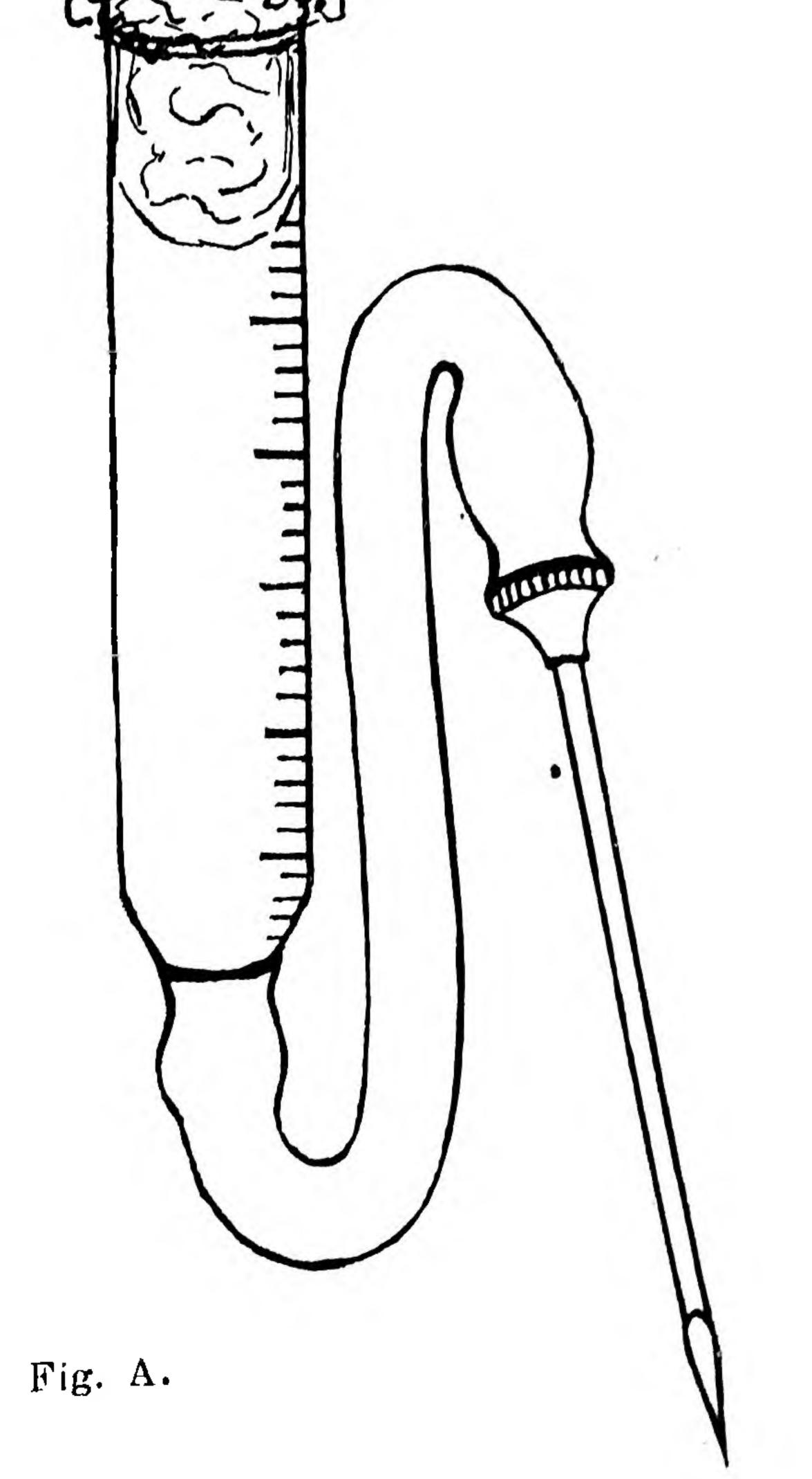
tubing, following exactly the same method as I did in case of the bulb of *Crinum asiaticum*. The glass tube was filled with a 25% solution of ferrous sulphate, a few drops of machine oil were poured on the surface of the solution to prevent evaporation, and the needle was kept on for a number of days, the solution getting in by means of a continuous upward pressure. The daily record of the quantity absorbed was kept by noting the level of the liquid. In the course of
