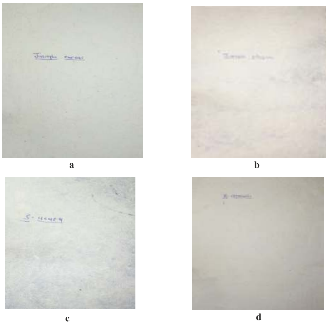
Figure 1: Sample papers produced from the studied materials (a) Jatropha curcas , (b) Jatropha podagrica , (c) Sida acuta and (d) Ricinus communis
