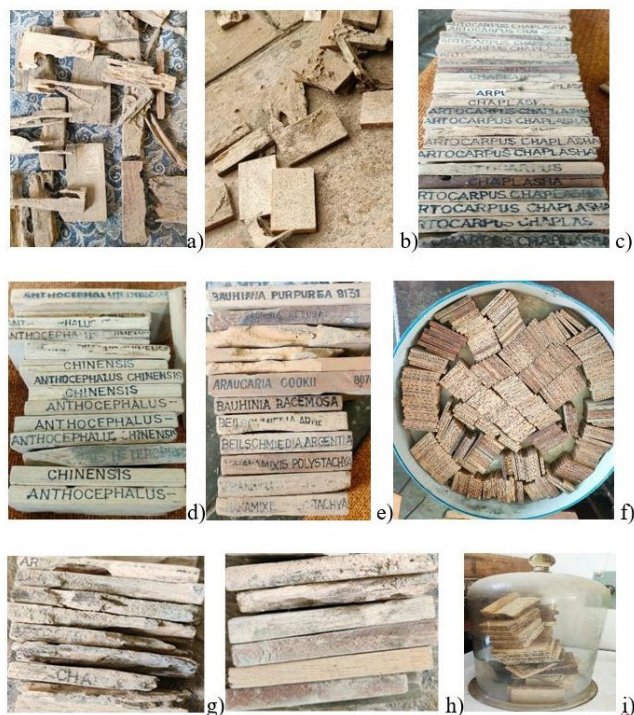
Figure 3 (a-i): (a),(b), Samples destroyed by termites c. Affected samples of Artocarpus chaplasha . d, e. Other affected Plant species f. Intact samples kept for fumigation g. Affected (marked) side of the samples h. Back side of the pic g, i.– Fumigating destroyed samples.
